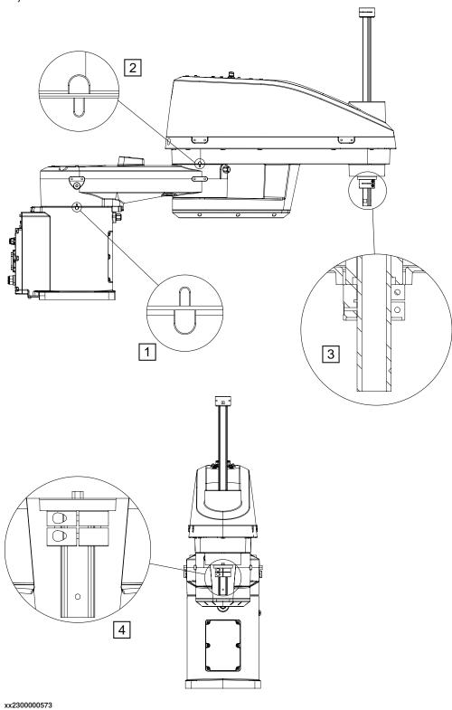
6.2.2 Calibration movement directions for all axes
