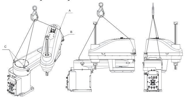
A: Sling may rub against the manipulator. Be careful to avoid damaging the painting surface. Better to use a buffer.
